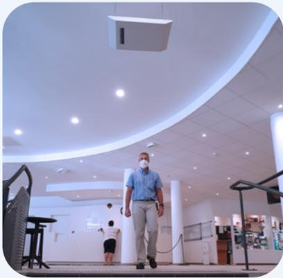
HID Textile Services' SPU500 is a high-performance EAS (electronic Article Surveillance) Station using RAIN RFID (UHF) technology. SPU-500 can be fixed above the entrance of the room, offering, in addition to item inventory, a discreet and efficient protection against theft. The specific antenna
